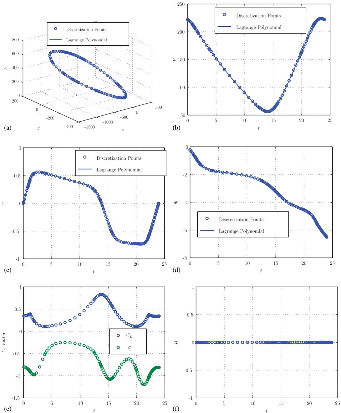
Figure 6. Solution on final grid for Example 3: (a) three-dimensional plot of  $(x, y, h)$ ; (b)  $V$  vs  $t$ ; (c)  $\gamma$  vs  $t$ ; (d)  $\Psi$  vs  $t$ ; (e)  $C_L$  and  $\sigma$  vs  $t$ ; and (f) Hamiltonian vs  $t$ .
