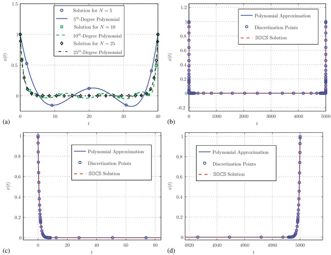
Figure 5. State solution for Example 2 with  $t_f = 40$  using global collocation and  $t_f = 5000$  using  $hp$ -adaptive pseudospectral method: (a) globally collocated solution for various values of  $N$ ; (b) entire state solution; (c) take-off segment; and (d) landing segment.
